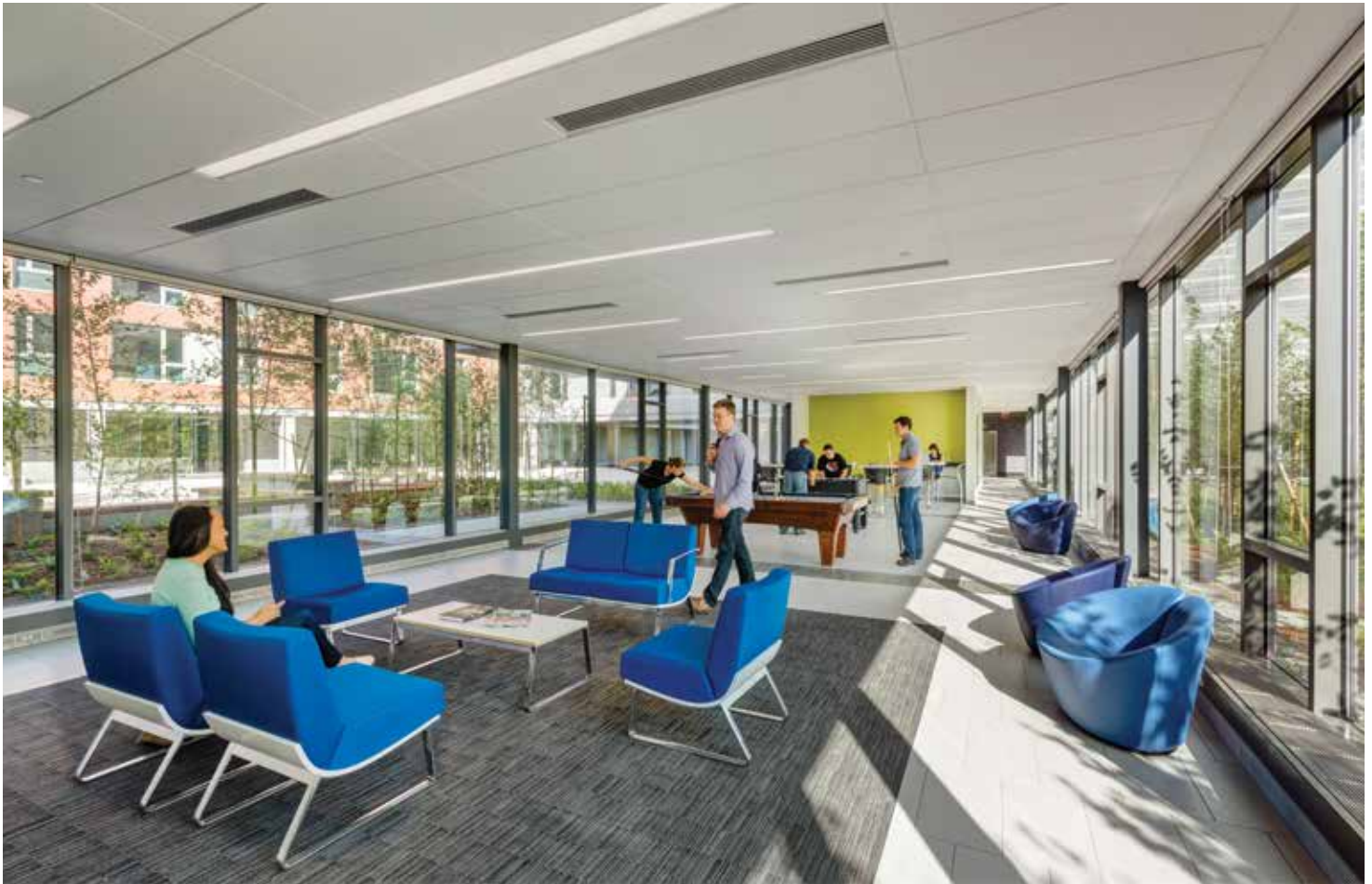
An aggressive lighting control system allowed Perkins+Will to combine ample daylighting with efficient LED and fluorescent technology to drop Weygang Hall's lighting power density 27% below the university's baseline.
