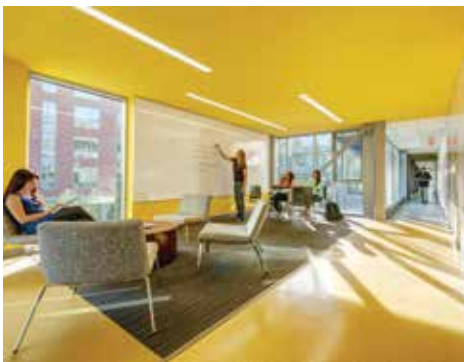
An aggressive lighting control system allowed Perkins+Will to combine ample daylighting with efficient LED and fluorescent technology to drop Weygang Hall's lighting power density 27% below the university's baseline.
